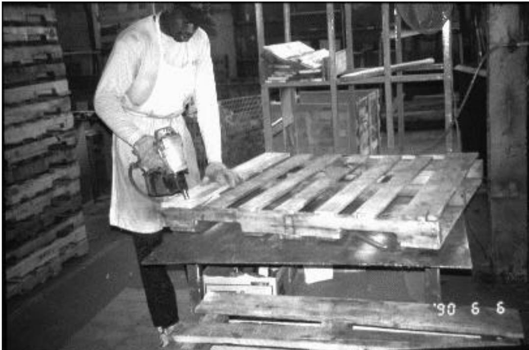
**FIGURE 7. A REPLACEMENT PART BEING USED TO REPAIR A PALLET.**
