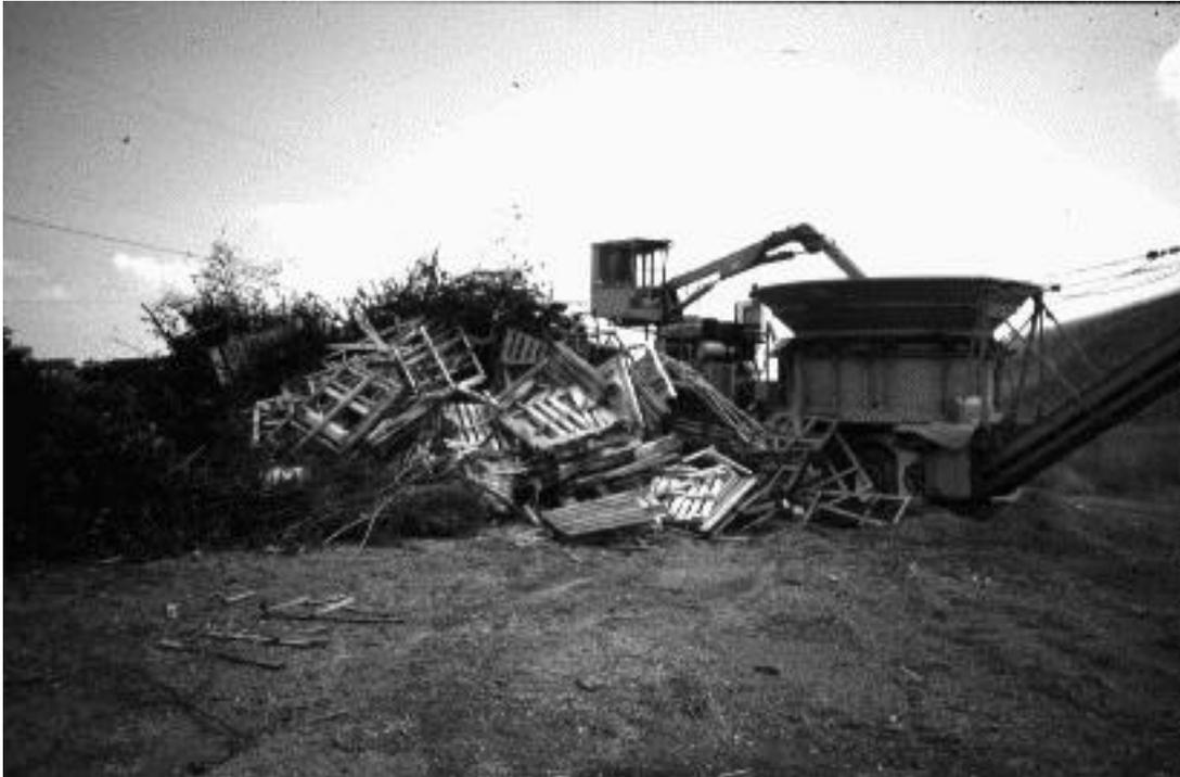
**FIGURE 8. CURRENT RECOVERY METHOD OF GRINDING PALLETS WITH TUB GRINDERS TO USABLE FIBER AT LANDFILL RECOVERY AREAS.**
